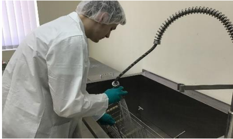
Glass cleaning with ultrasonic wave & deionized water
