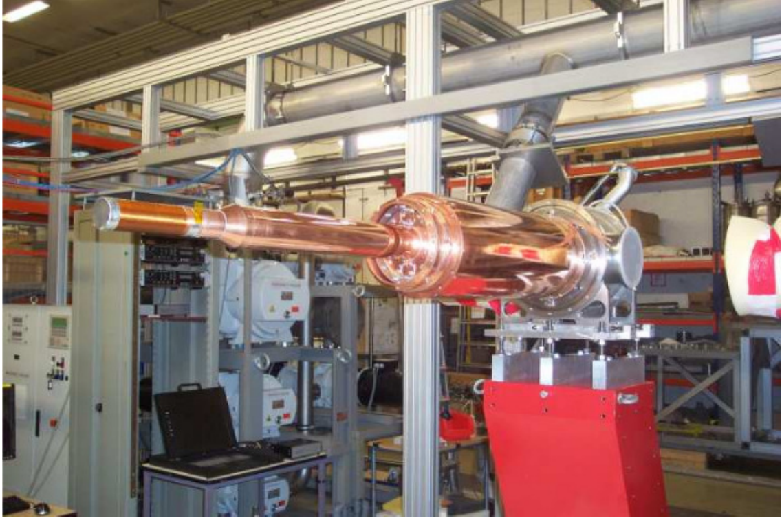
Figure 7: The new dilution refrigerator for the Crystal Ball frozen spin target.
