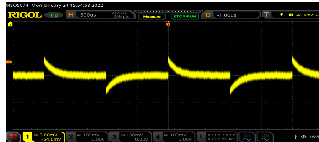
Output signal at 500Hz and 10mV input amplitude
