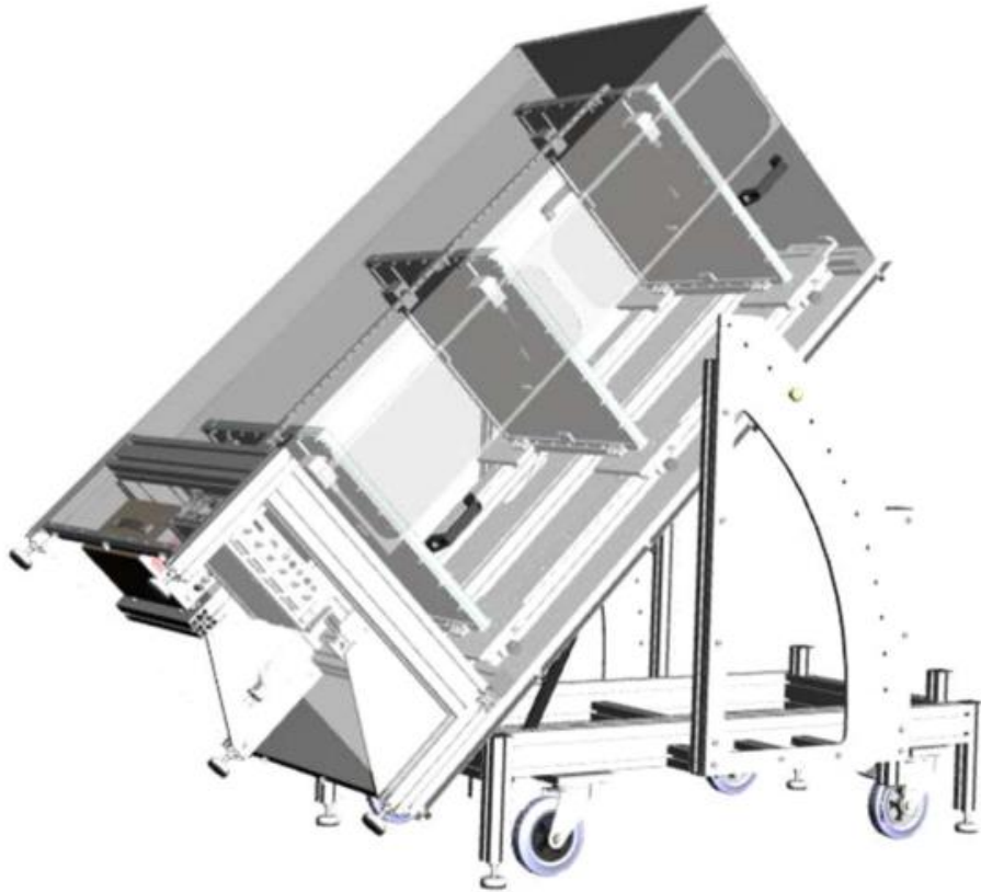
Fig. 2. Design of the WatTo telescope, represented here with only three detectors.
