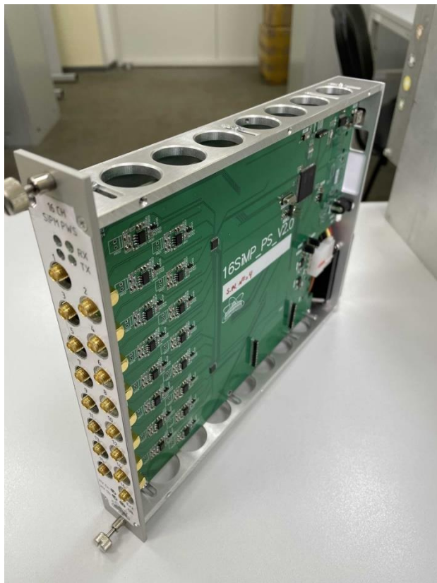
A view of the power supply module
