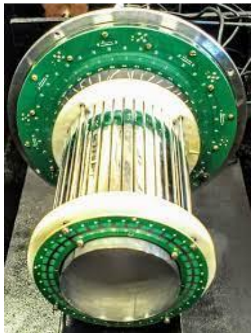
A view of barrel detector strip assembly with SiPMs board
