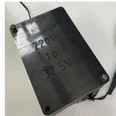
A view of the external transformer power supply
