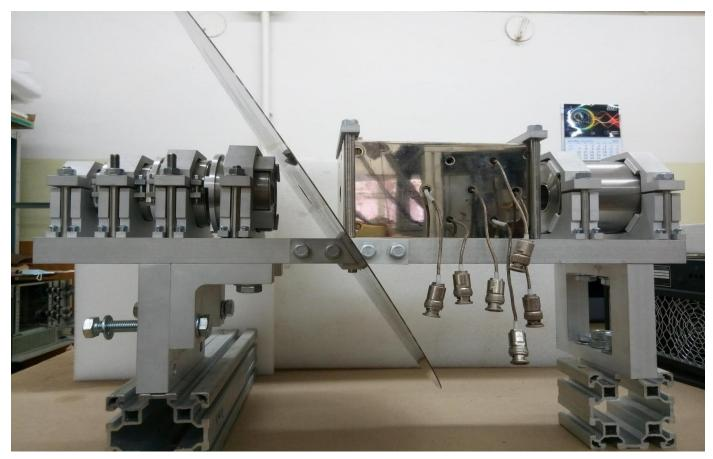
This device designed to separate atoms from a beam by their electron and nuclear spins. It consists of:
