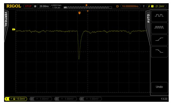
To measure single photoelectron mode we cover photocathode with a black cloth.
