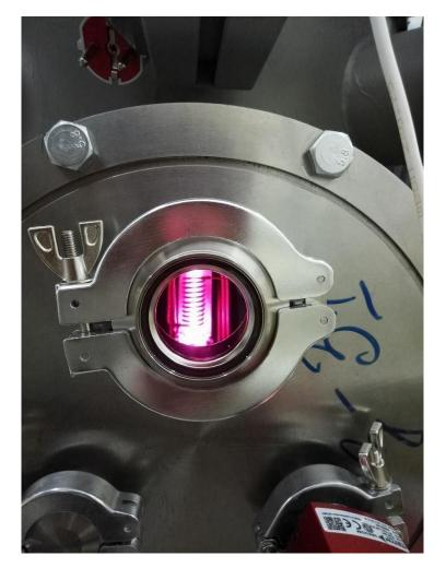
Pyrex glass pipe on the left called a "Dissociator". High frequency inductor wound around it. Inductor powered by 280 watts with 13 MHz frequency. This induces a HF discharge that makes a dissociation of molecules.
