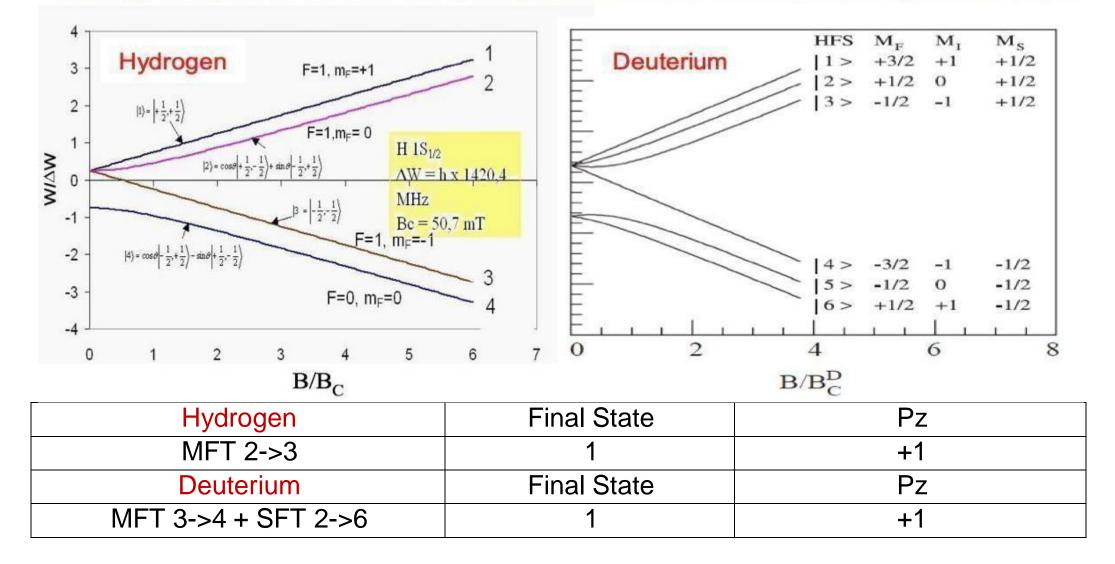
To obtain polarization in APol we will use following MFT and SFD for Hydrogen and Deuterium.
