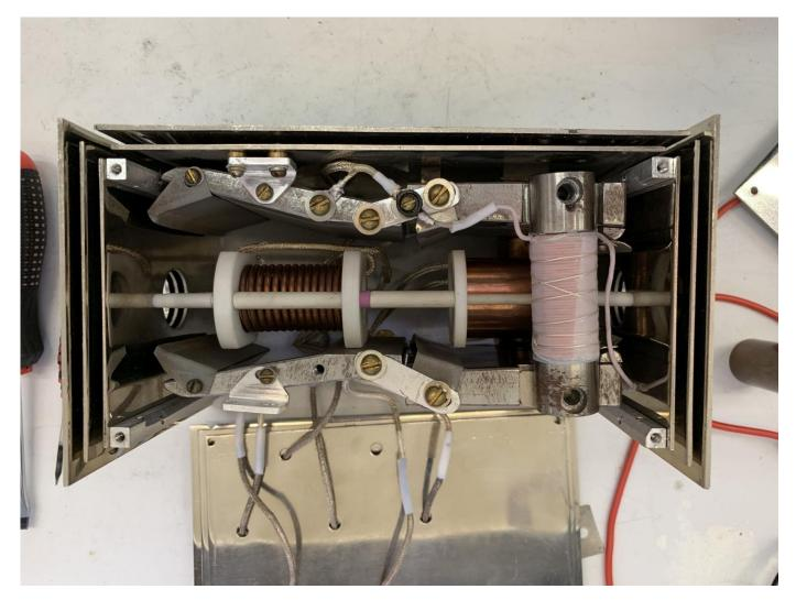
Medium field transition (MFT) cell is need to obtain maximal polarization of atoms. To achieve this **nuclear spins should be co-directed to their electronic spins.**
