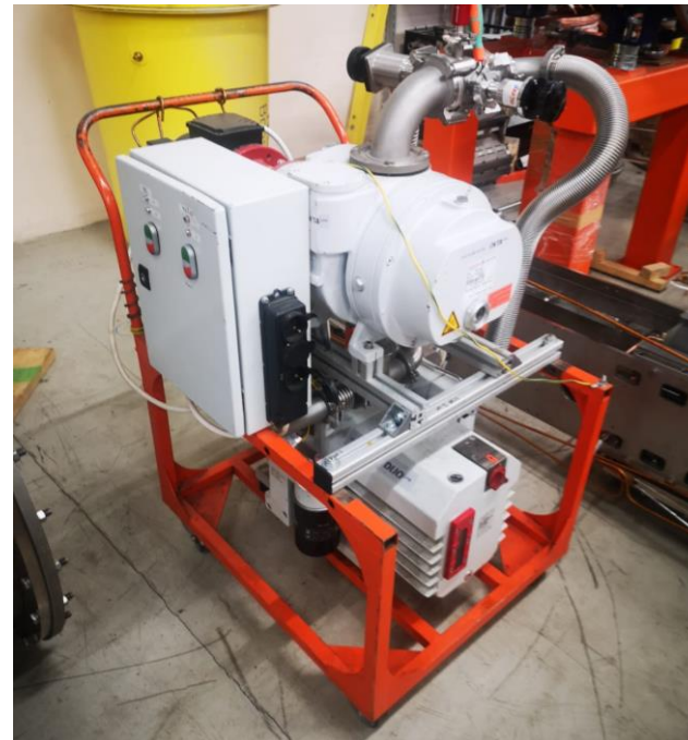
Diffusion vapor pump and pumping station with two foreline pumps
