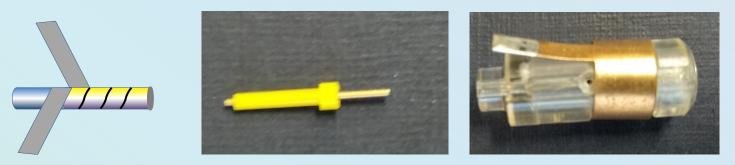
Twisted structure of the straw tube. The picture illustrates a winding on a precision rod. The end-plug and the crimping pin are used to fix the anode signal wire
