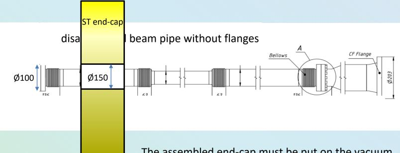
The outer diameter of the beam pipe is 100 mm without flanges. Central hole in end-cap is 150 mm and defined by a beam pipe The assembled end-cap must be put on the vacuum beam pipe, together with the rest of the internal detectors
