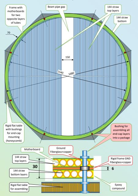
One coordinate layer consists of a frame on which 288 individual straw tubes are glued on both sides
