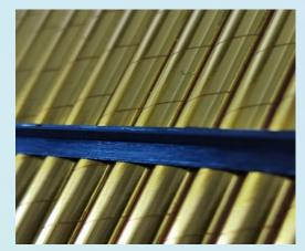
Carbon fiber strips used as external support for the straw tubes.
