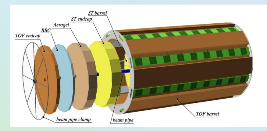
The end-caps of ST, Aerogel, BBC, and TOF are mounted one-by-one by moving them along the beam pipe
