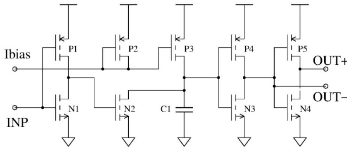
Differential version of the stretcher has been adapted from PADI ASIC stretch cell (IEEE Transaction on NS, April 2021, PP(99):1-1)
