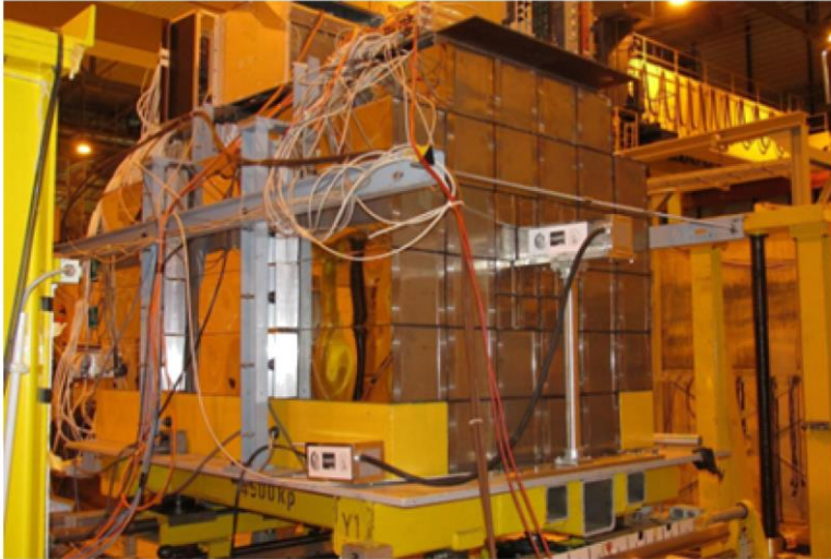
Photo of the PSD placed on the beam line downstream of the NA61/SHINE detector
