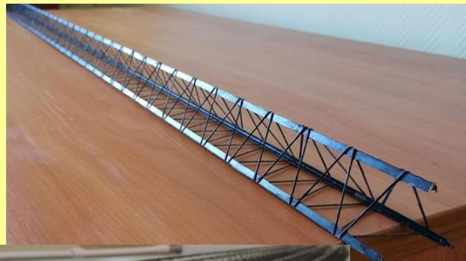
1) The technology of production of Extra Lightweight Detector Support Structures was modified for Russian prepreg «НИИКАМ-PC/M55» (Research Institute of Space and Aviation Materials)
