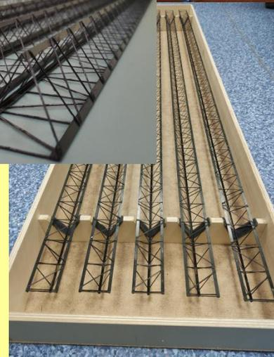
30 Wound-truss structures were produced at SPbSU and shipped to JINR
