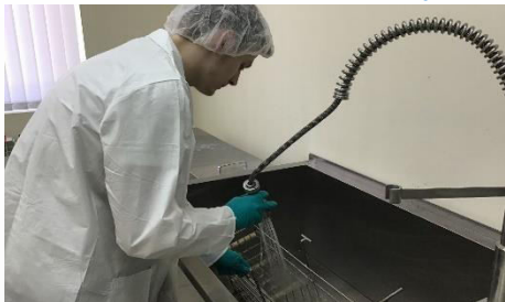
Glass cleaning with ultrasonic wave & deionized water
