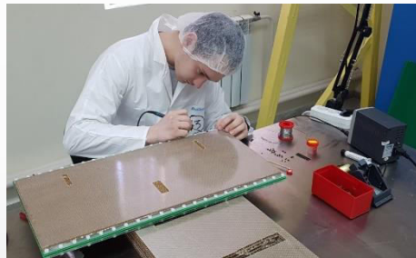
Soldering HV connector and readout pins
