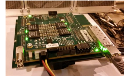
The readout electronics: FPGA based 64 channel ADC64 board, 62.5MS/s (AFI Electronics, JINR, Dubna).
