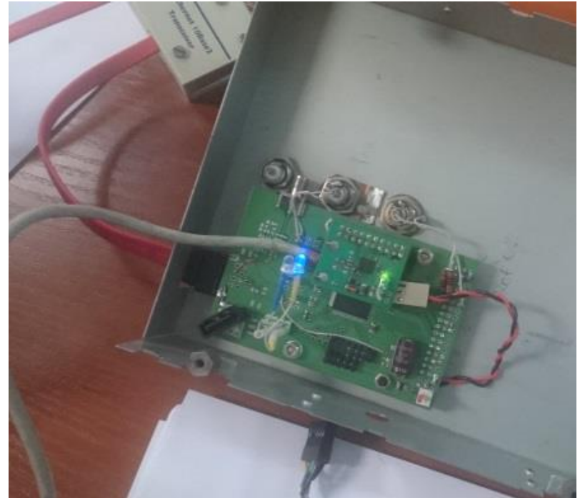
Fig.34. Photo of the device of the two-channel fast electronics module based on discrete comparators. Work is in progress.
