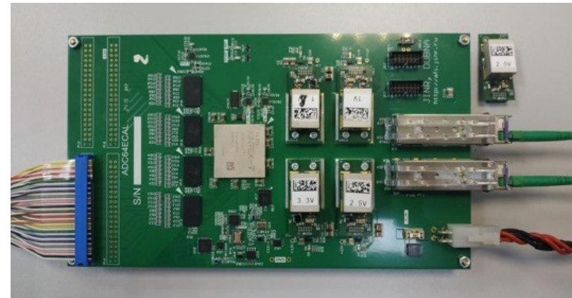
ADC64ECAL under test, passive air cooling
