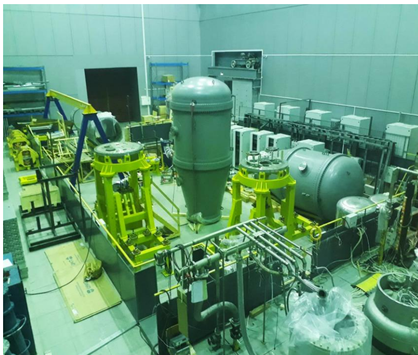
Fig. 14. Assembly of the collider electron cooling system at BINP.
