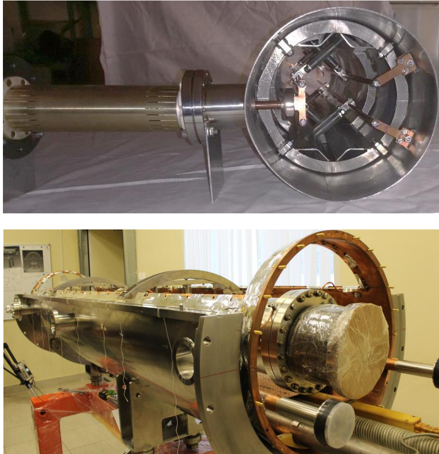
Fig.2 Nuclotron injection kicker: design of the electrodes (upper photo), assembly in the vacuum chamber (bottom photo).
