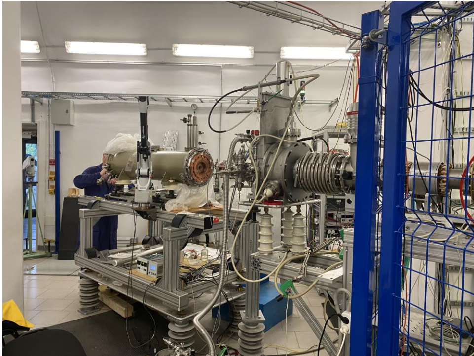
Fig. 12. KRION-6T mounted on the High Voltage platform
