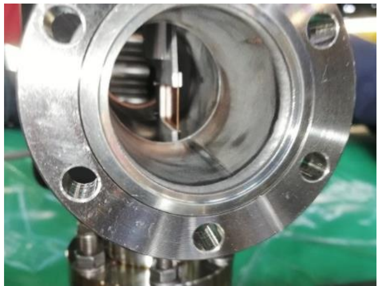
Fig. 11. Stripping station (left) and the stripping foil inside the vacuum chamber (right).
