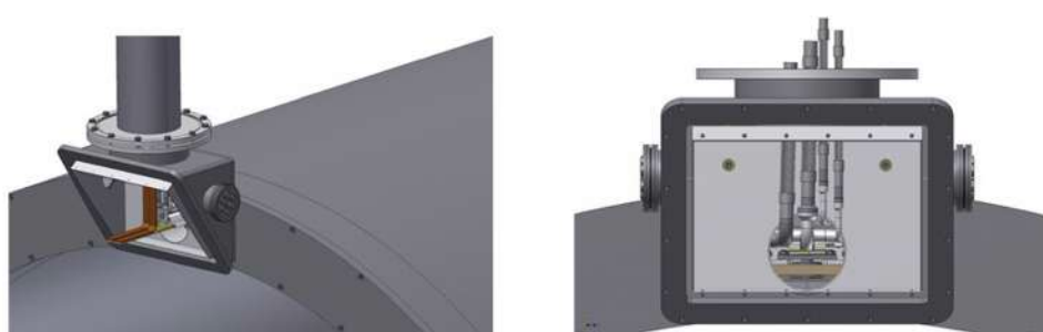
Figure 5.32: Connecting bus-bars and process pipes into the Interface box.
