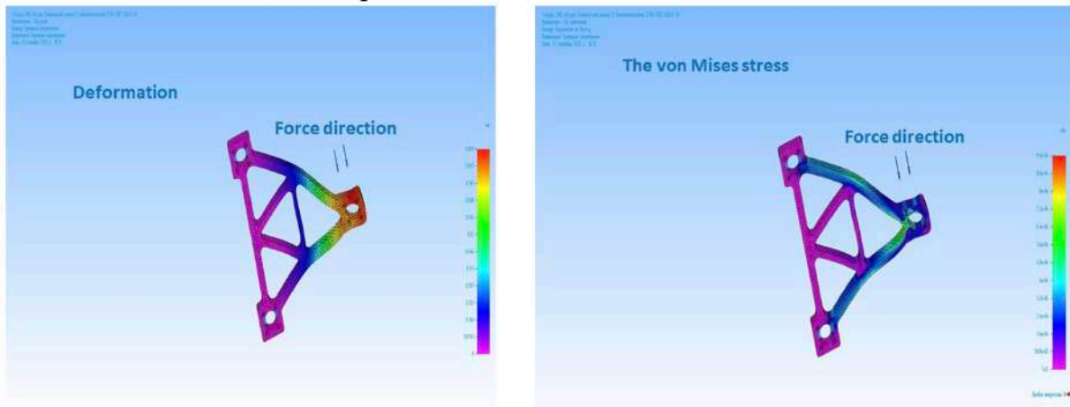
Figure 5.23: Calculated mechanical loads on the triangle support.
