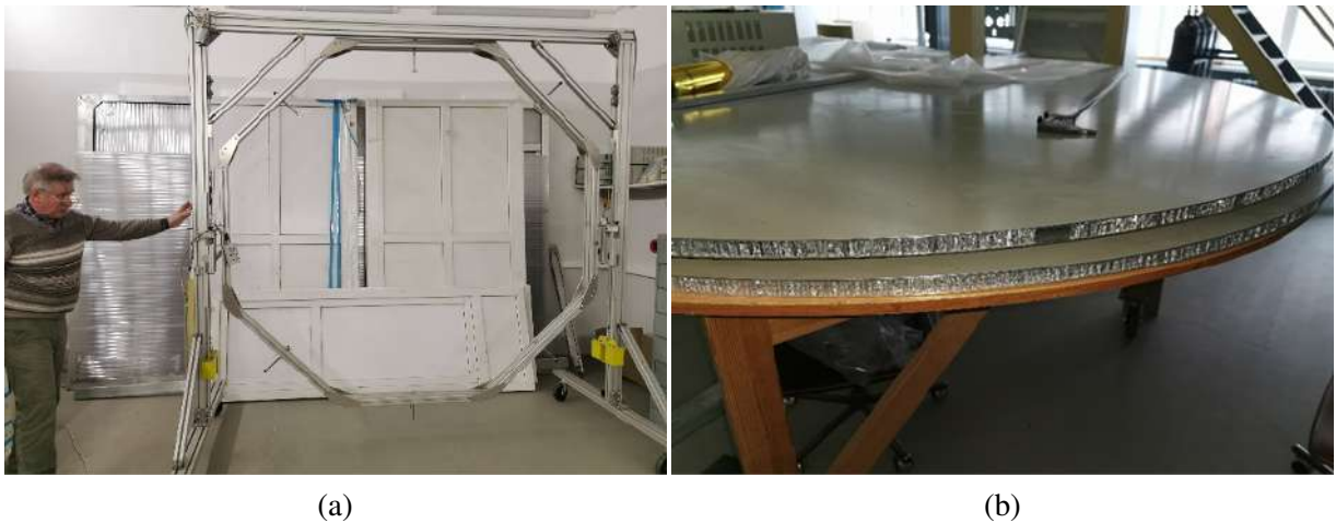
Figure 9.39: (a) Technological equipment for assembly. (b) Octagonal rotary platform and a portable honeycomb board for assembling are shown. The diameter of the portable board is 2300 mm, the thickness is 50 mm.
