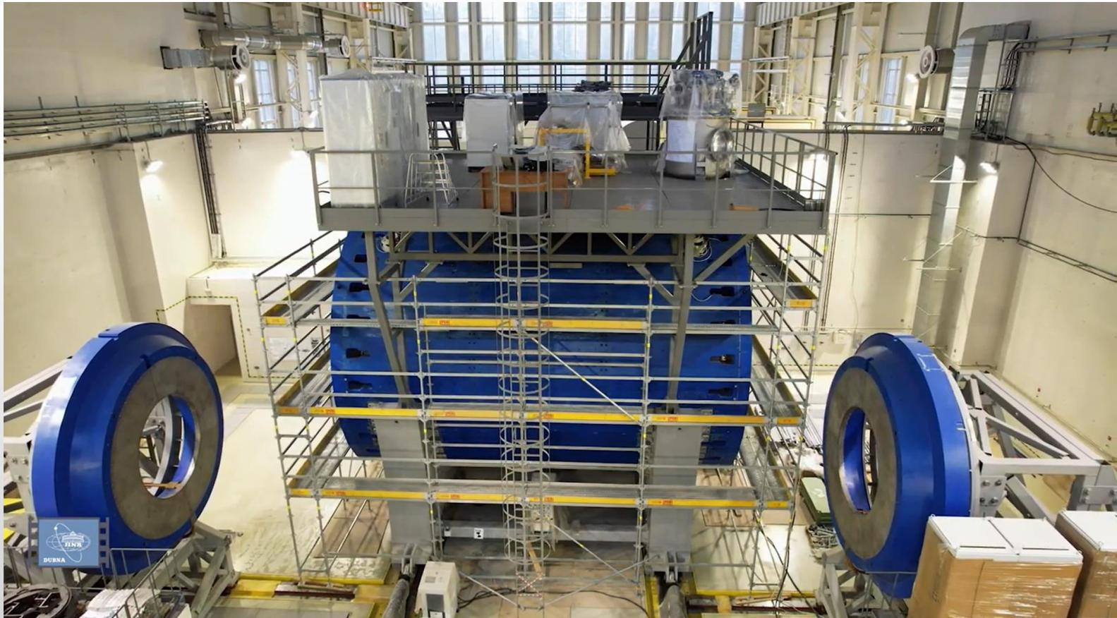
❖ One of two experiments at NICA collider to study heavy-ion collisions at  $\sqrt{s_{NN}} = 4-11$  GeV
