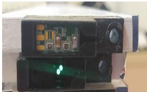
Sketch of the strip with SiPM board and housing. The real look of the SiPM PCB inserted to the housing
