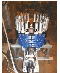
measuring angular and energy distributions of emitted  $\gamma$ -rays and neutrons in (n,n') reactions with neutrons at the energy of 14 MeV.
