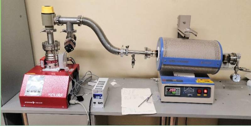
Vacuum oven 1000 degrees Celsius for sample annealing
