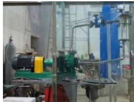
loop test for windowless HML target
