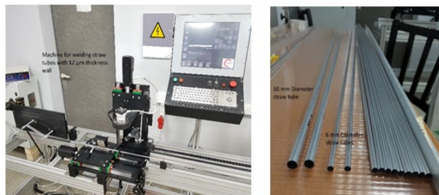
Fig. 23. Left: Welding machine; Right: 9.8 mm and 6 mm straw tubes.
