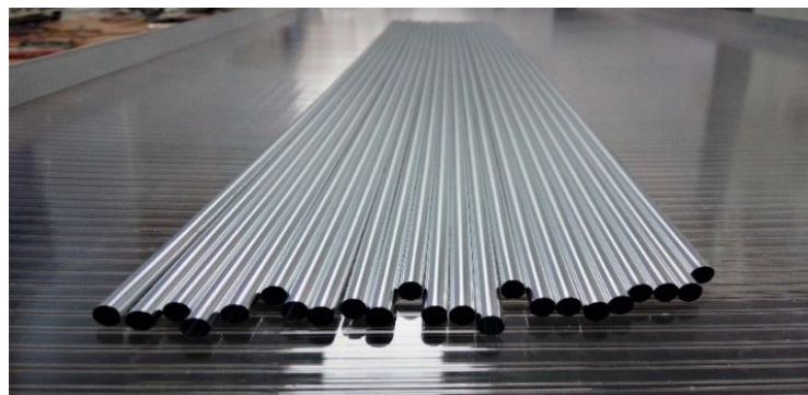
Fig. 27. New straw tube with 5 mm diameter for JINR detector prototype.
