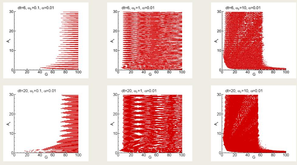
Here we present the  $(G, A_s)$ -plane diagram for different values of the normalized frequency of the magnetic resonance  $\omega_F$  and the current pulse time interval  $\Delta t$ . The results are obtained with G-stepsize  $\Delta G$ =0.1,  $A_s$ -stepsize  $\Delta A_s$ =0.1 at r = 0.1;  $t_0$  =25.
