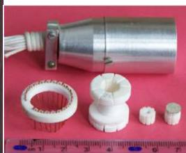
Surveillance specimens in Rostov NPP reactor vessel
