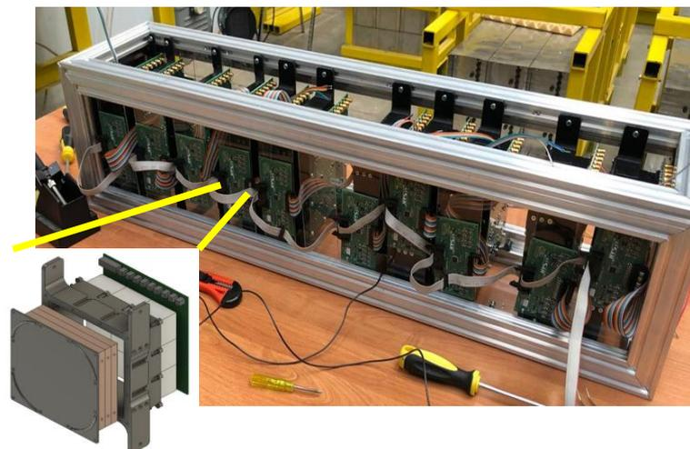
HGN prototype (15 layers, thickness  $> 2 \lambda_{int}$ ):
