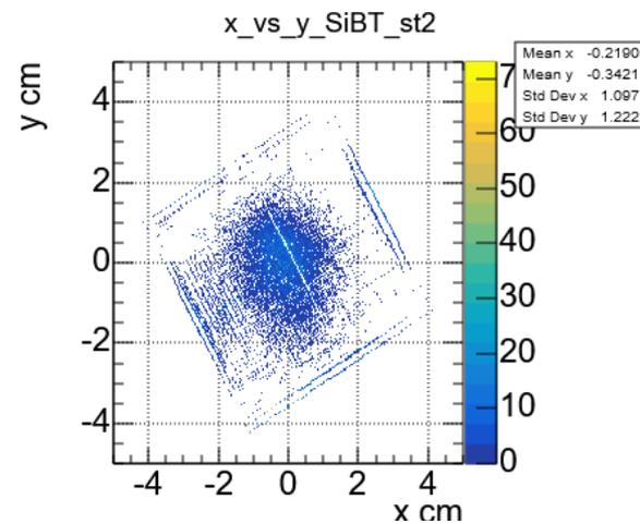
Measured beam spot at target
