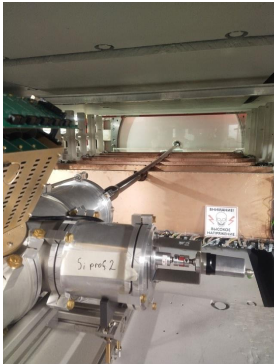
The position of the carbon beam pipe with installed lower GEM detectors
