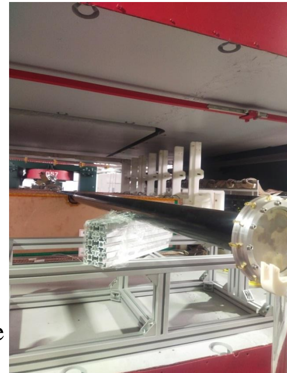
The position of the carbon beam pipe with installed lower GEM detectors
