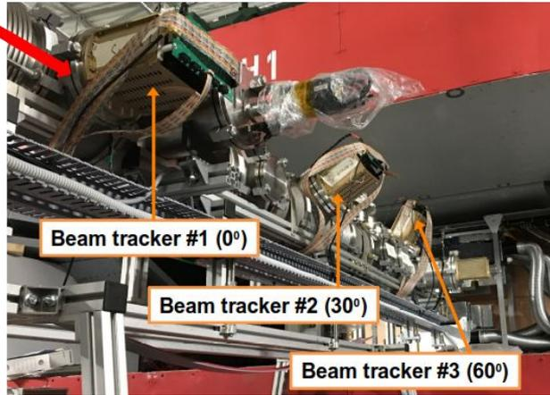
Si detector inside vacuum chamber
