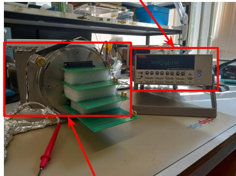
beam tracker and boards to read the current from each strip
