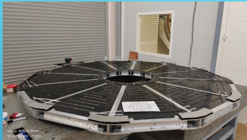
Service wheel with thermal panels (12pc)
