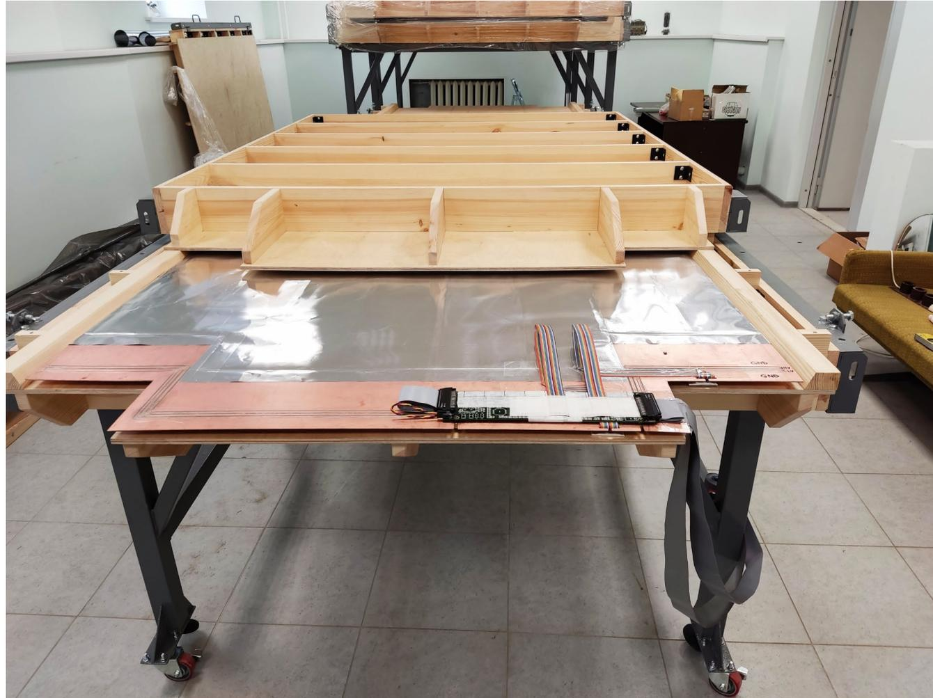
Detecting plane mockup (MDTs, strip board, analog FEE cards and cables) inside the slot 30 mm of stand-imitator: **rather dense space !**
