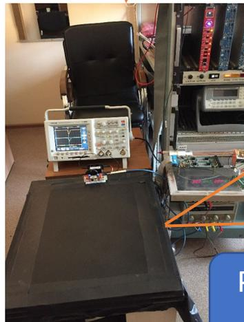
Position of cosmic trigger counters (top/bottom) at RS prototype
