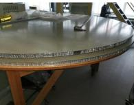
The straw planes are assembled on a rigid **honeycomb board** on a rotatable octagonal frame
