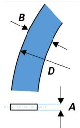
The detector frame should be 100 mm wide (B) and will be made of carbon fiber
