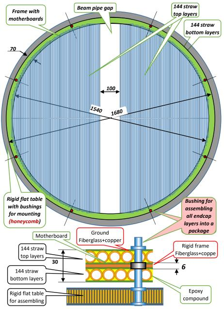
One coordinate layer consists of a frame with 288 straw tubes, 9 (32 ch) motherboard. Straw are glued on both sides Straw endcap Proposal
