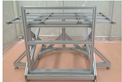
Fig. 16. Stand for quadruplets assembly.
