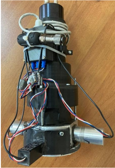
Fig. 5: Muon trigger system and its testing at TUM.
