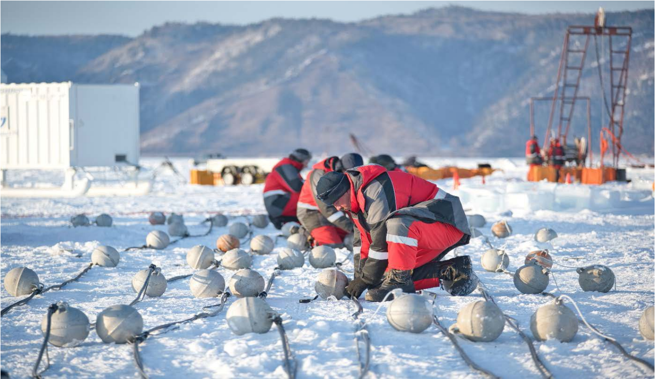
Figure 3: Assembling the Baikal-GVD installation cluster garland.
