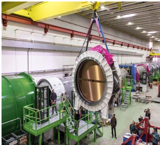
Figure 10. Installation process for one of four straw chambers in the NA62 experiment.
