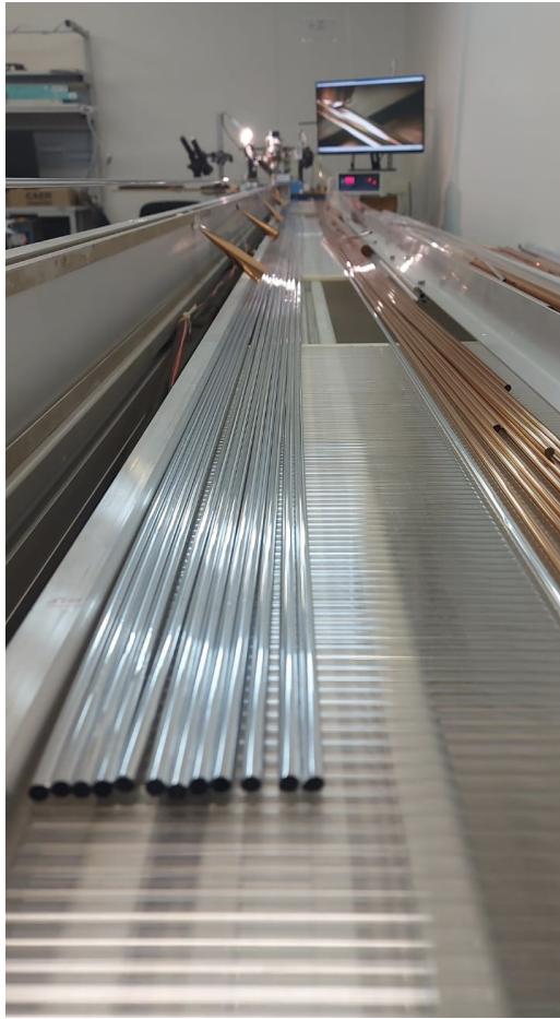
Figure 11. 5m long straws for STT prototyping produced at JINR.
