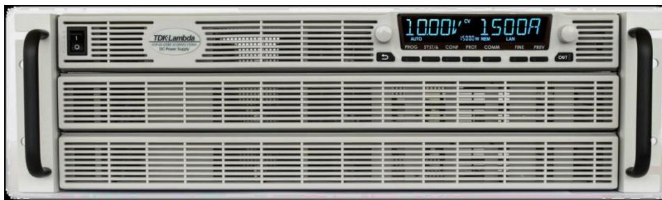
The current control resolution of 20ppm is provided by the internal ADC resolution, which for this family of sources is 16 bits. This means that with the sufficiently high external feedback loop gain, accuracy and stability of the external current sensor of at least 20ppm, it is possible to provide a long-term stability of the 5200A current source of 20ppm.
