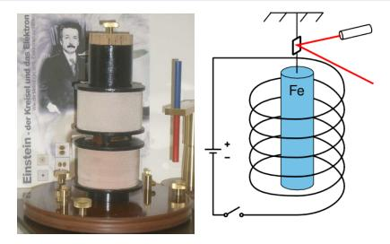
Electron spins get aligned in external magnetic field which is compensated by rotation of the ferromagnetic material.
