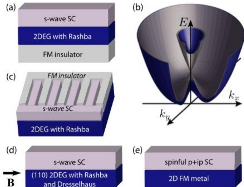
**Figure 9.** (a) A 2DEG with Rashba spin–orbit coupling can effectively realize a topological 2D ‘spinless’  $p + ip$  superconductor when in contact with a ferromagnetic insulator and conventional s-wave superconductor. (b) Band structure for the 2DEG when time-reversal symmetry is present (gray) and with a non-zero Zeeman field (blue) that opens up a ‘spinless’ regime. (The break in the spectrum appears for clarity.) Alternative devices that support topological phases appear in (c)–(e).
