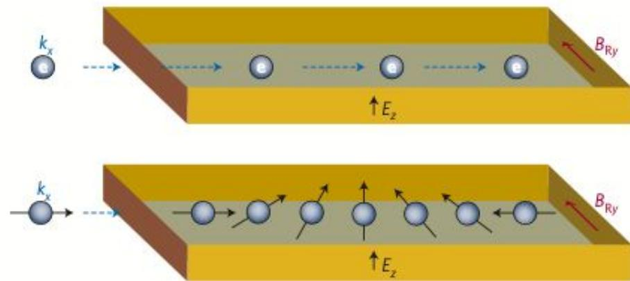
**Inverse spin galvanic effect and spin precession.** Top: Moving electrons ( $k_x$ ) with a perpendicular electric field ( $E_z$ ) experience the Rashba field,  $B_{Ry}$ . Bottom: In a Rashba system, the spin of the moving electrons (arrows) precesses around the axis of the Rashba field.
