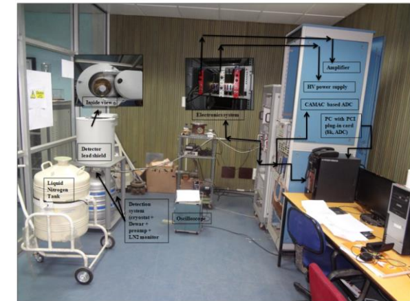
Fig. 3 Experimental set-up for the offline \gamma -ray spectroscopy using HPGe detector system.
