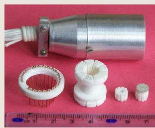
**Surveillance specimens in Rostov NPP reactor vessel**
