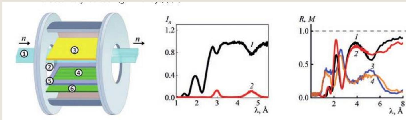
Ionization chamber (1 — neutron beam; 2 — input and output windows; 3 — cathode; 4 — grid; 5 — mesh frame; 6 — anode) for measuring intensity of reflected neutrons (1) and charged particles (2) from Cu(10nm)/V(55nm)/CoFe(5nm)/6LiF(5nm)/V(15nm)/glass. Neutron reflection coefficient (1,2) and the coefficient of secondary radiation (gamma-rays) (3,4).
