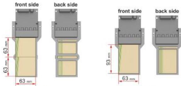
**Si-module with two double-sided strip sensors of  $63 \times 63 \text{ mm}^2$  each**     **Si-module with one double-sided strip sensor of  $63 \times 93 \text{ mm}^2$**
