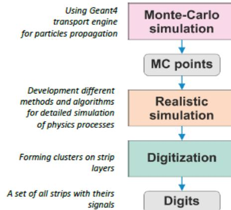
**Complete simulation** for detectors comprises the following stages:
