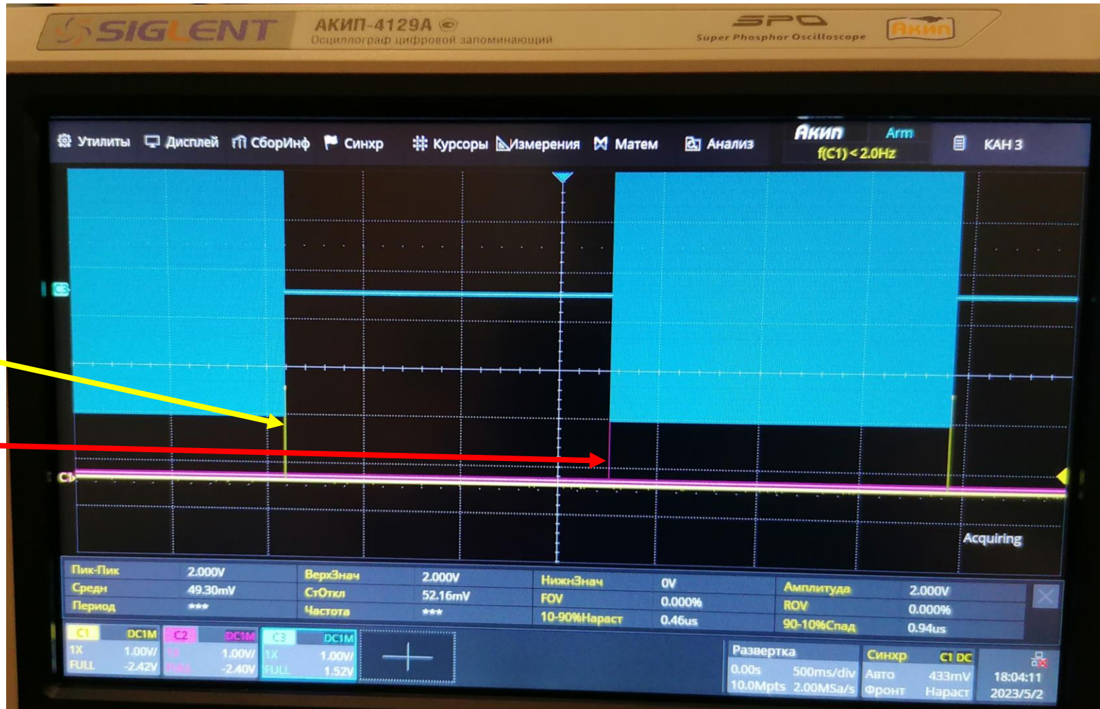
Figure 7. Oscillogram of an incorrect frequency.
