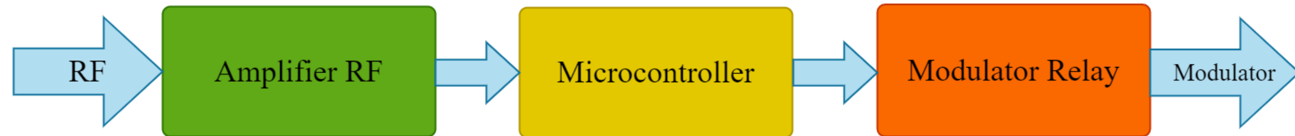
Figure 3. Block diagram of the frequency protection.
