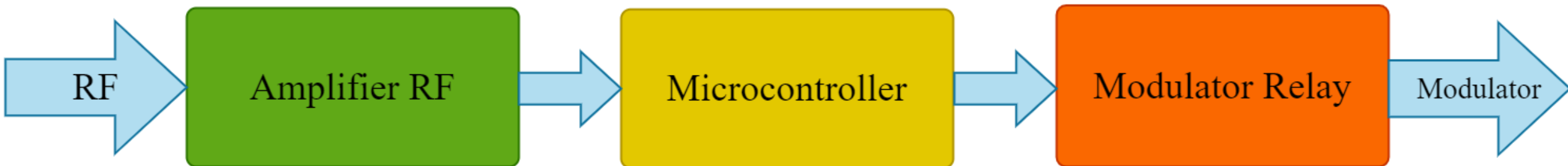
Figure 3. Block diagram of the frequency protection.
