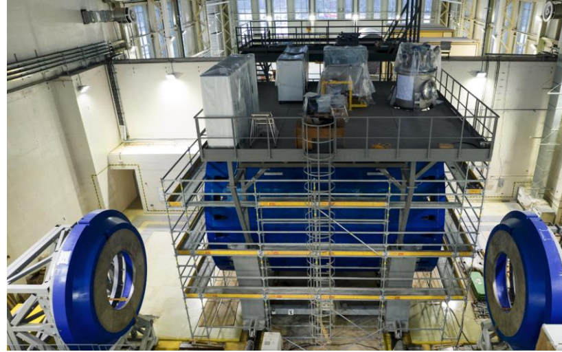
The magnet consists of Solenoid inside Iron Tokes and two correction coils inside of Endcaps
