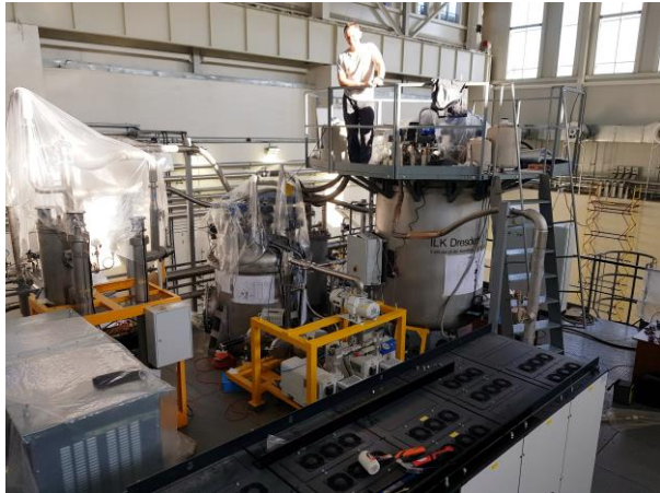
Cryogenic platform with Satellite refrigerator and Control Cryostat
