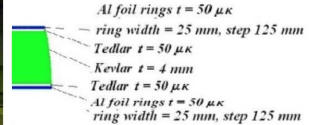
$D_{\text{in}} = 2660 \text{ mm}, L = 3400 \text{ mm}$
