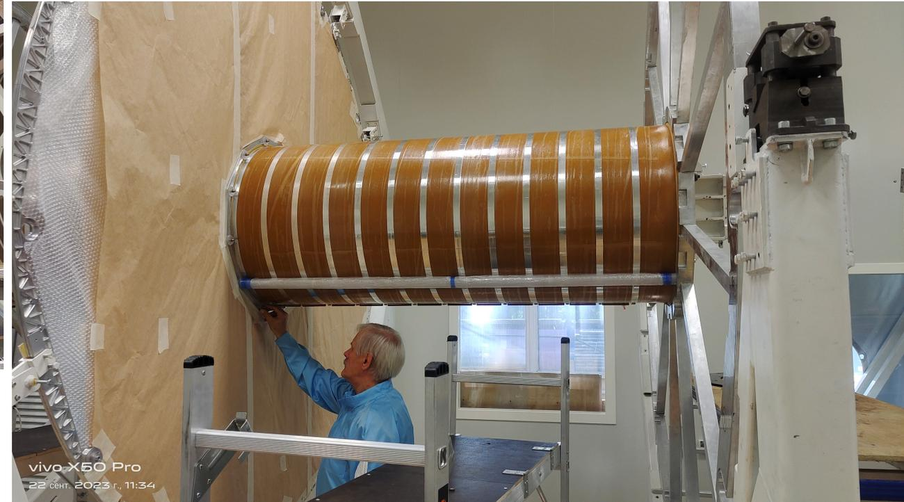
Inner field cage rods installation
