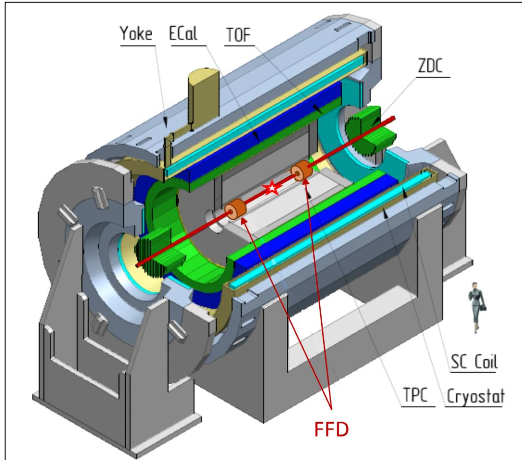
Two Cherenkov subdetectors  $FFD_E$  and  $FFD_W$  has 20 modules & 80 cells each with position at 140 cm from MPD center
