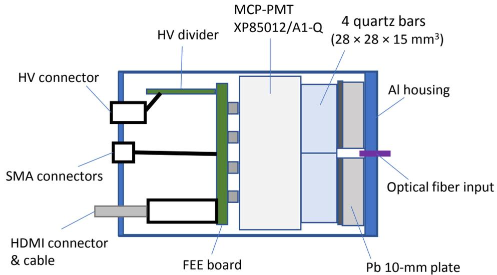
FFD module size:  $64 \times 64 \text{ mm}^2$
