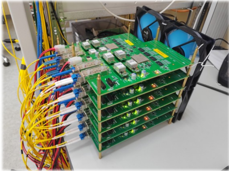
ADC64ECAL under test, active air cooling
