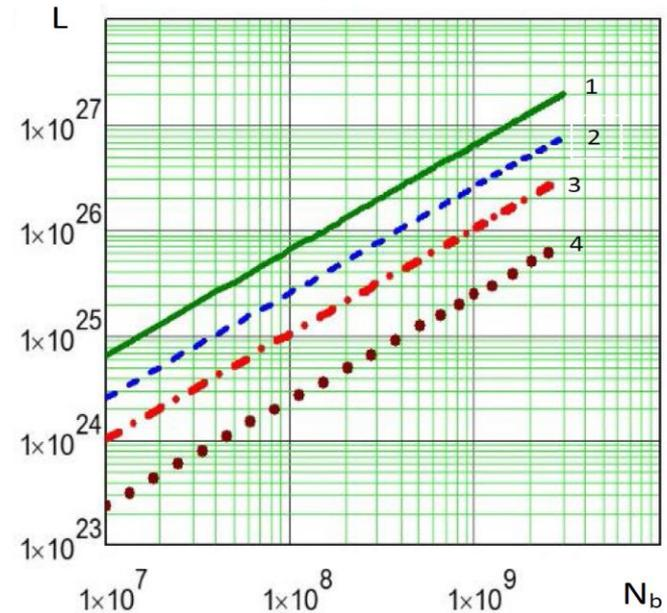
**Dependence of luminosity on number ions per buch at different energies (1) 4.5 GeV/u (2) 3GeV/u, (3) 2 GeV/u, (4) 1 GeV/u.**
