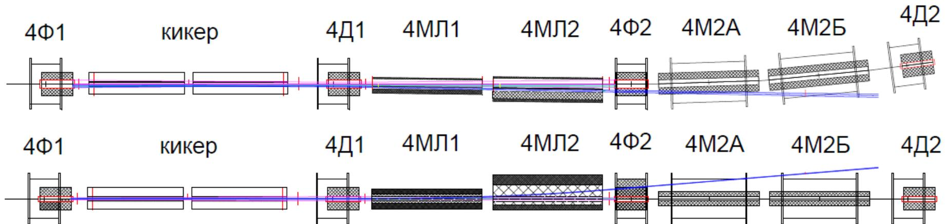
**Application of one extraction Lambertson magnet permits to reach the maximal kinetic ion energy 2.5 GeV/n in first Collider beam runs**
