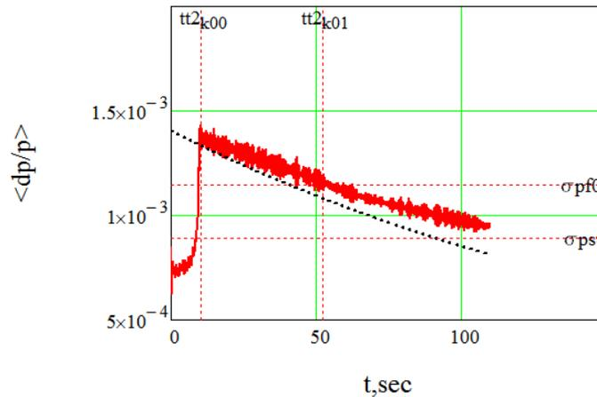
Dependence of bunch length and momentum spread on time at cooling time of 100 s.
