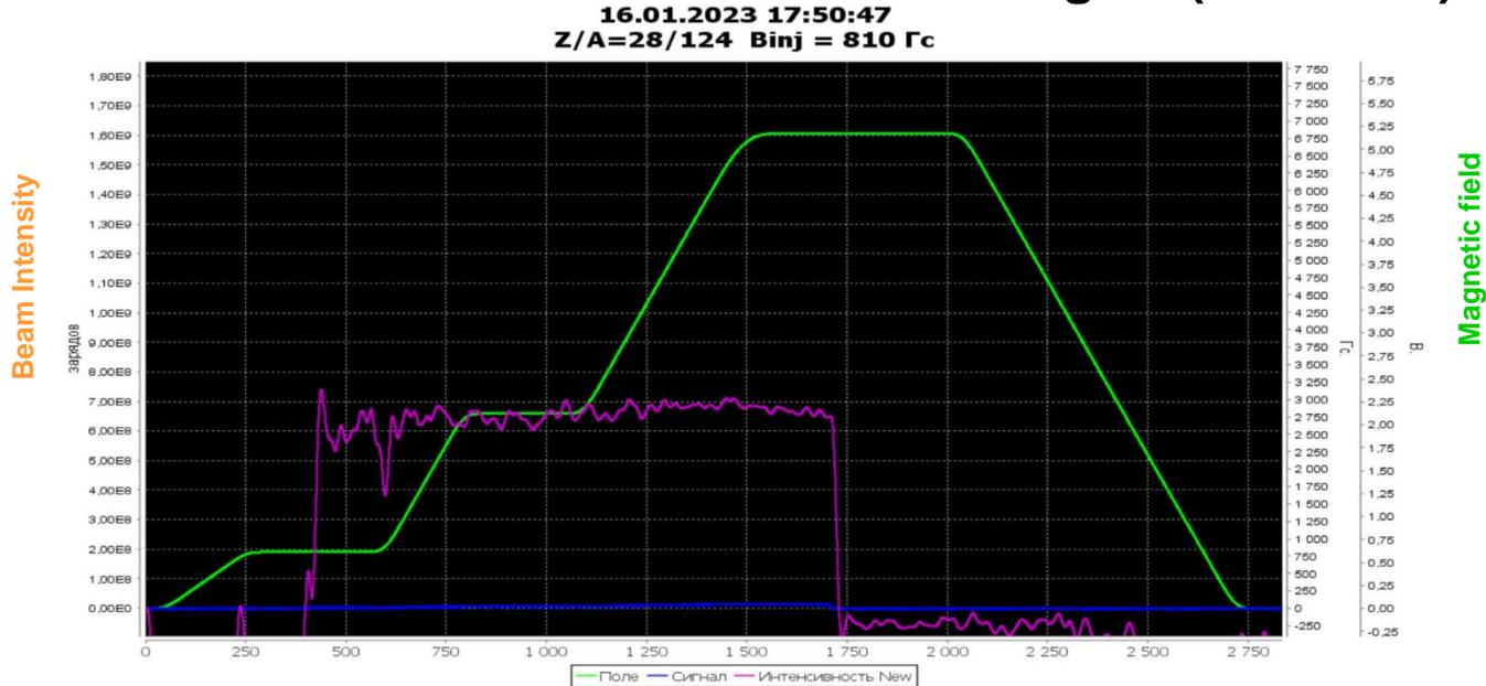
Booster-Nuclotron run - September 2022 - February 2023 for BM@N baryonic matter researches. Booster acceleration of ions  $^{124}\text{Xe}^{28+}$  to energy 204,7 MeV/n, where they were stripped up to bare nucleus end extracted in Nuclotron.
