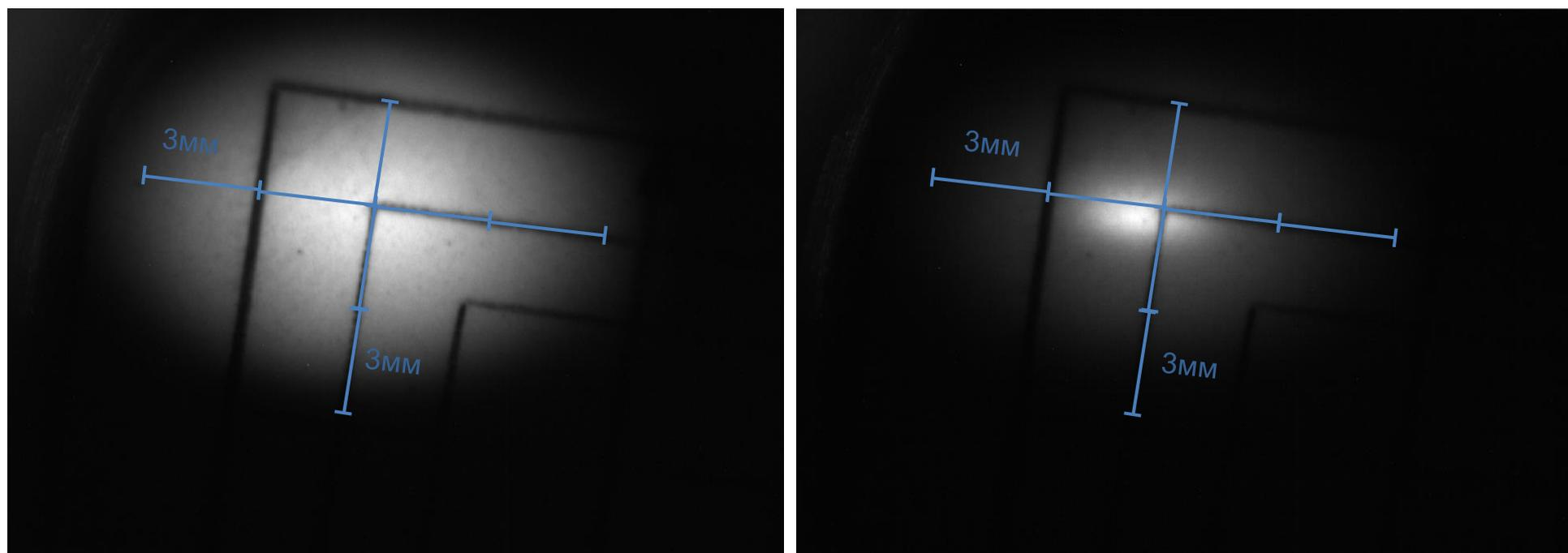
Image of electron beam at Nuclotron entrance without cooling and with cooling.
