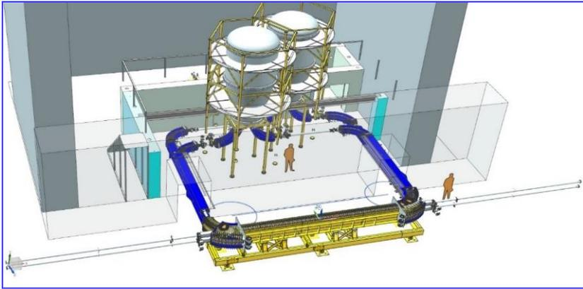
HV Electron Cooler for NICA Collider
