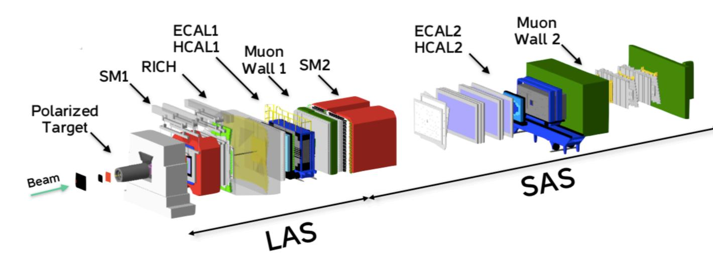
COMPASS is a high energy experiment which studies hadron structure and spectroscopy with high intensity pion and muon beams. The experiment is located at the M2 beam line of the Super Proton Synchrotron at CERN.
