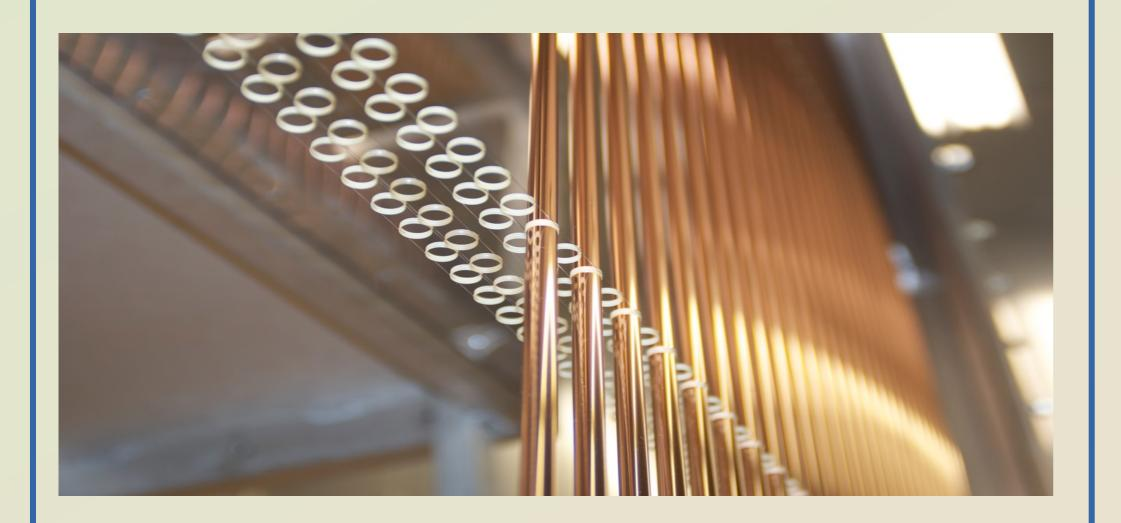
Track coordinates are reconstructed according to the measured signal arrival time defined by the drift time of primary electrons from the track to the anode wire. A number of operating and future experiments use Straw Tube detectors for precise tracking such as ATLAS TRT[1]. Example of successful operation of a large area Straw Tube Tracker made of straws produced by ultrasonic welding method: the NA62 [2] detector.
