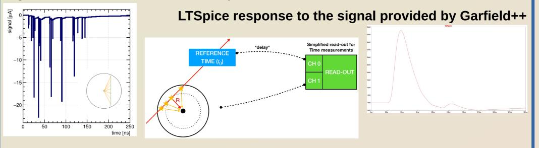
The signals obtained within Garfield++ simulation. Then this signal was processed by LTSpice. (LTSPICE is one of the best software for analysis and design of electronic schemes. It is an easy to use, widespread, and free product with very good convergence). Once the signal is processed by LTSpice one can use it for further analysis.
