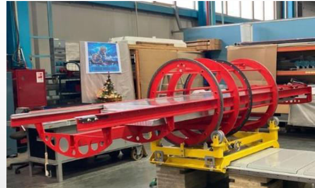
TOF installation bench in LHEP
