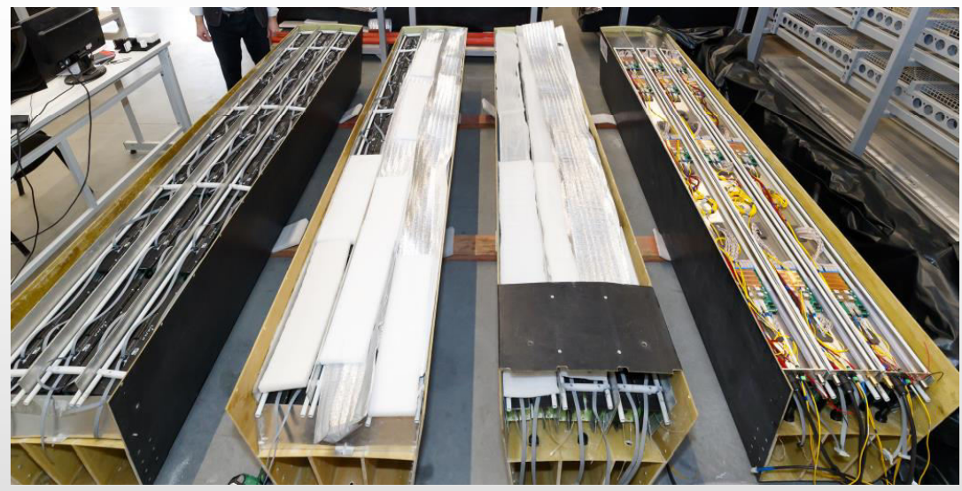
Half-sectors at different stages of assembly
